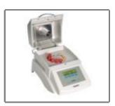
The HT200S with its high speed digestion technology meets the need for fast, effective digestion in municipal, industrial, and service laboratories. The HT200S heats in maximum 8 minutes and cools down in 13 minutes. The actual analysis can start after just 35 minutes and the pure digestion time is only 15 minutes.
